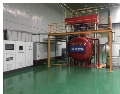
图17 国产6缸独立加压大型扩散焊设备 Fig.17 Domestic large diffusion bonding furnace with six independent cylinder
